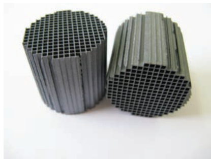
Figure 20.15 High cell density (300 cells in -2 ) SiC based monolithic structures for future deployment as HYDROSOL reactor supports.
