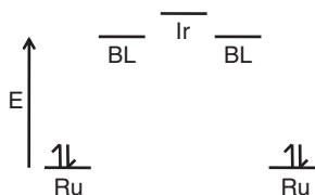
Figure 19.9 Orbital energy diagram for Ir centered supramolecular complex, [\{(bpy)_2Ru(BL)\}_2IrCl_2]^{5+} (BL = 2,3 bis(2 pyridyl)pyrazine (dpp), 2,3 bis(2 pyridyl)quinoxaline (dpq), or 2,3 bis(2 pyridyl)benzoquinoxaline (dpb)).
